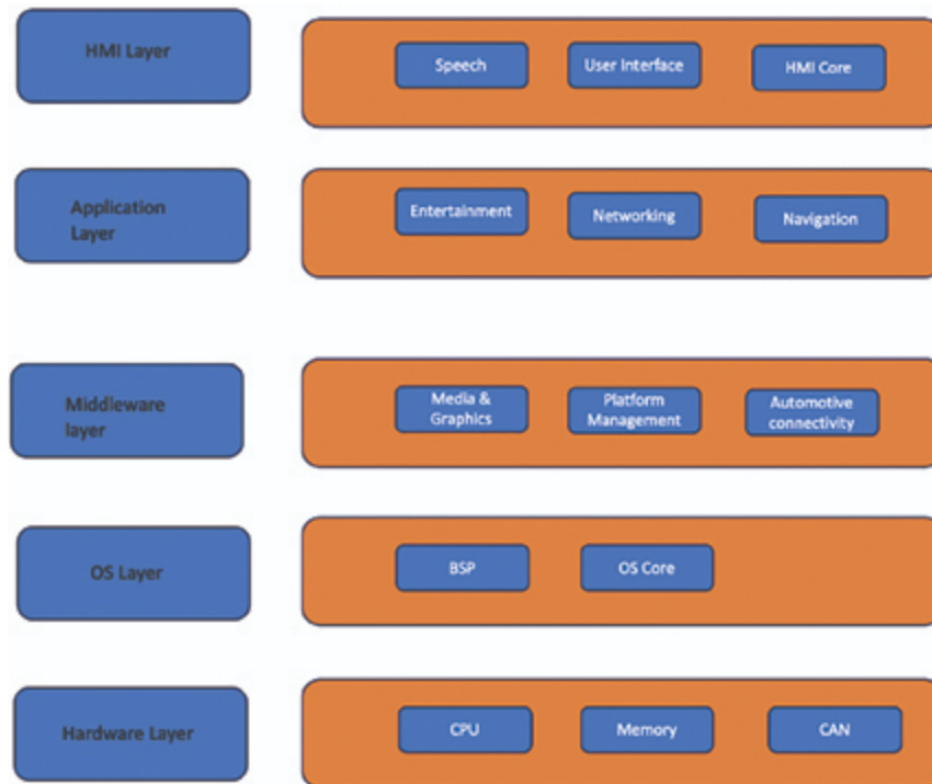
Figure 1.1: Understanding the Infotainment Components
