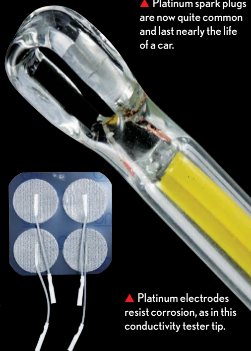
▲ Electrodes for delivering therapeutic electrical pulses to the skin can also be made of platinized thread.
