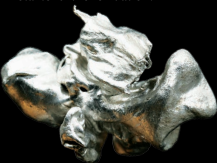
▲ Nodules created by pouring molten aluminum into a bucket of water.
