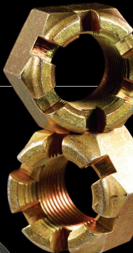
▶ Treatment with dichromate gives these cadmium-plated castle nuts a gold color.
