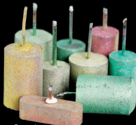
▶ Pressed tantalum powder capacitor cores.
