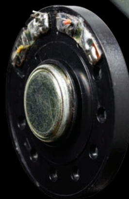
▲ Neodymium magnets are crucial in lightweight hi-fi headphones.
