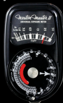
▼ Selenium photocells were widely used in photographers' light meters.
