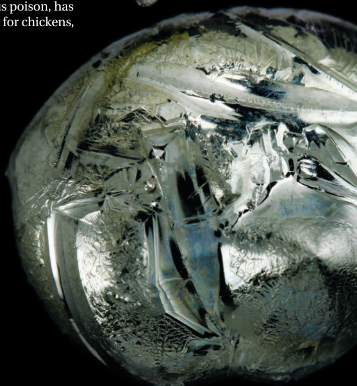
▼ Molten germanium forms crystals on the surface as it cools.
