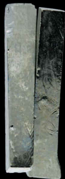
◀ Bulk commercial germanium is sold in ingot bars: This is the broken end of one, showing the internal crystals.
