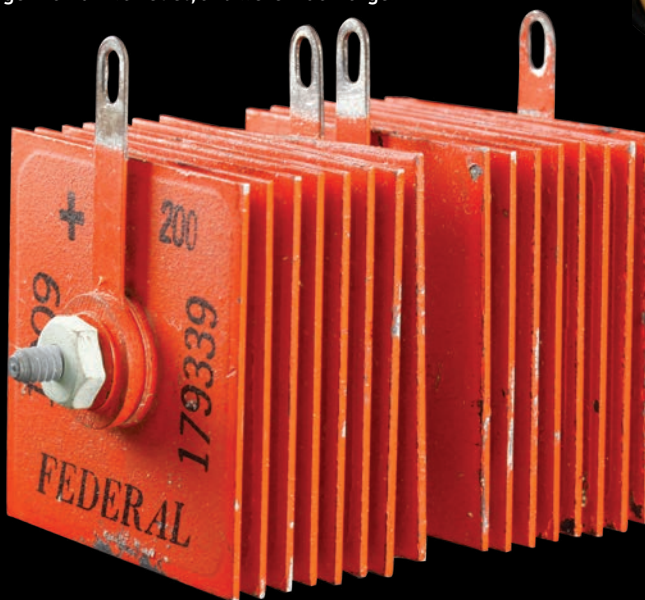
▼ Selenium rectifiers (diodes) predate silicon and germanium varieties, and were much larger.
