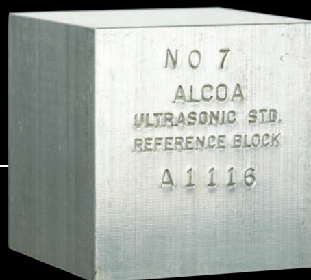
▲ Solid block of aluminum for testing purposes.
